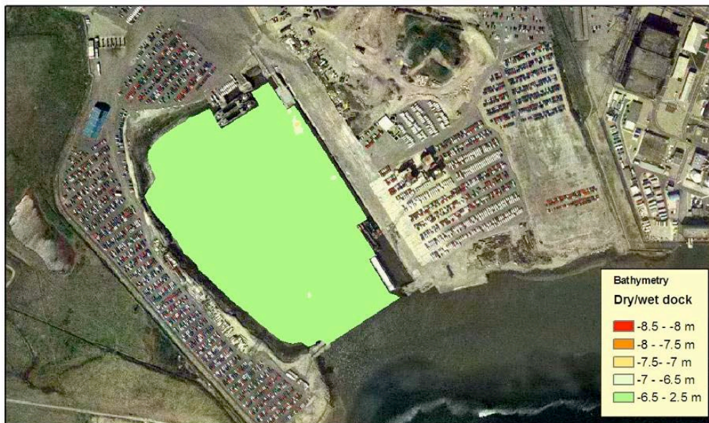
Figure 3-6 Detailed bathymetry for dredging of Dry/wet dock
