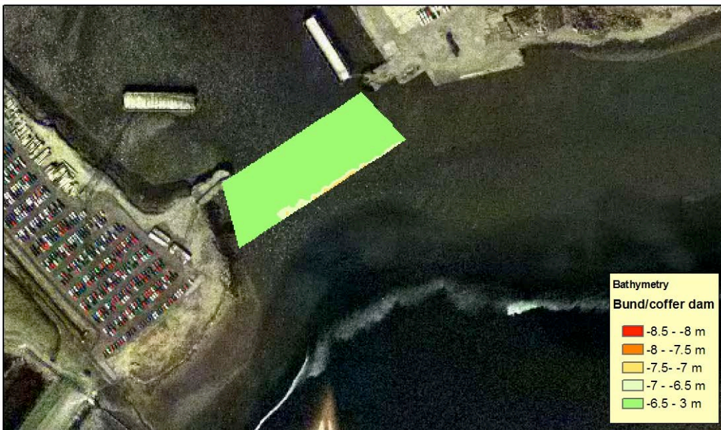
Figure 3-5 Detailed bathymetry for dredging of Bund/cofferdam area
