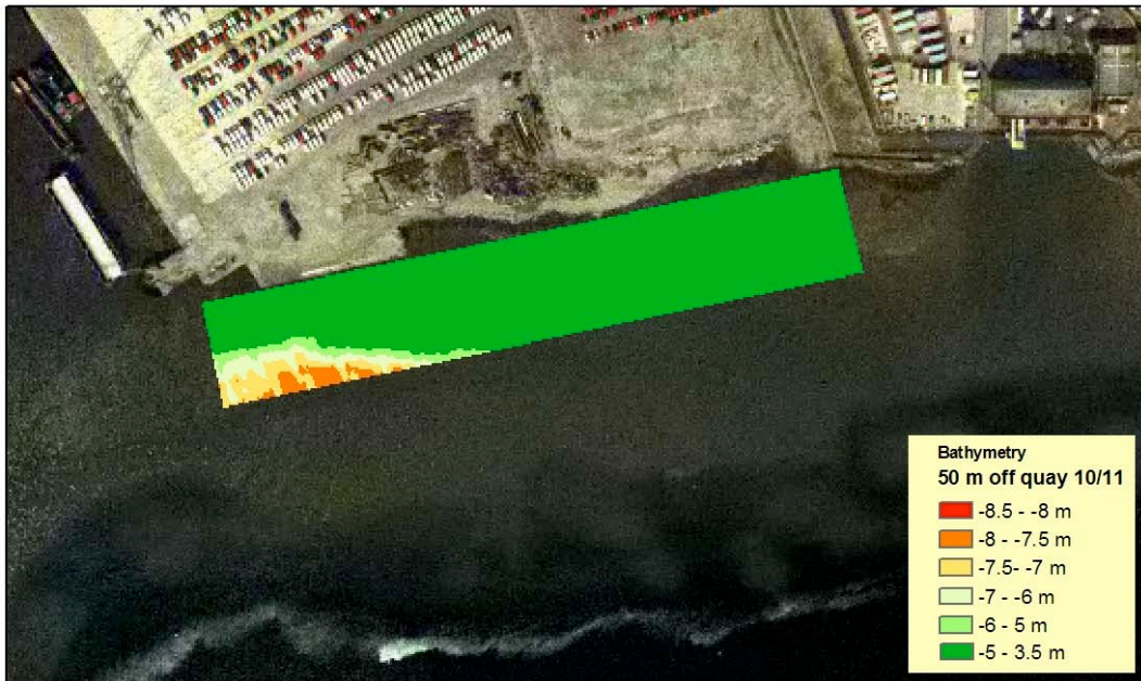
Figure 3-4 Detailed bathymetry for dredging of Quay 10 and 11
